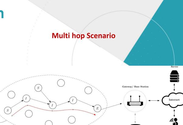
S: IoT Source node I: IoT Intermidate node E: IoT End node
