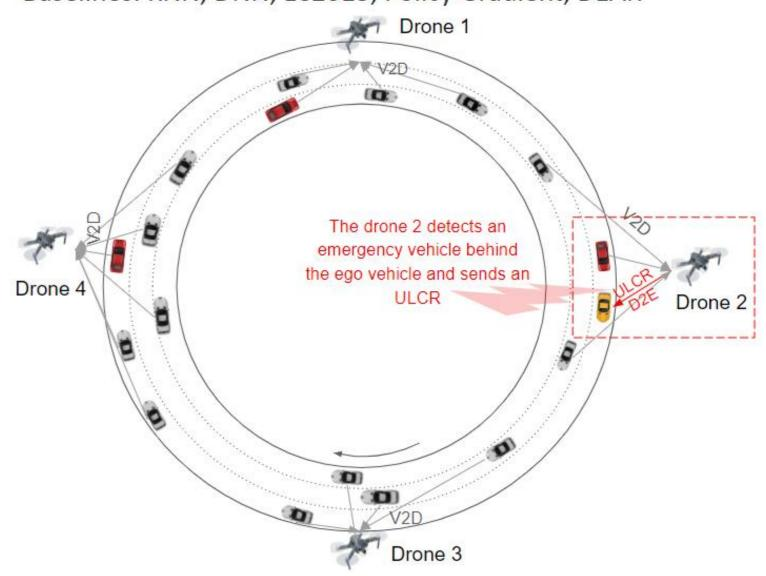
V2D: vehicle-to-drone communication D2E: drone-to-ego communication
