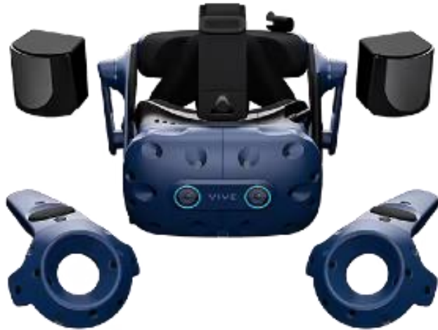
HTC Vive Pro Eye Integrated Tobii eye-tracker
